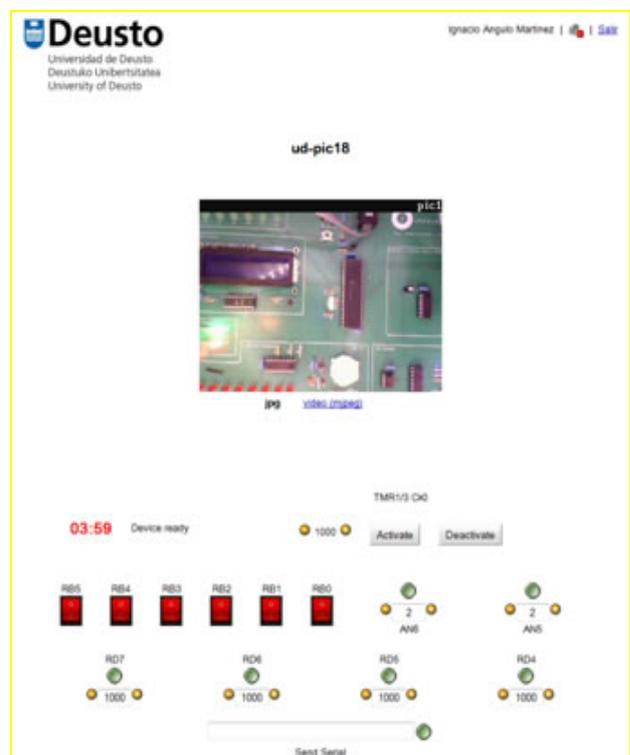
Figure 5. WebLab Deusto PIC Interface.
