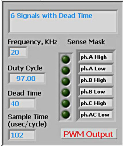
Figure 6. LabVIEW Inverter PWM Diagnostic Window
