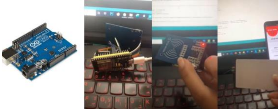
Fig. 4. Arduino Uno Microcontroller, Card reader and RFID card
