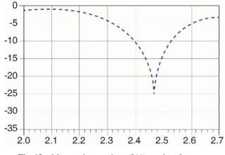
Fig. 13. Measured return loss (S11) results of antenna
