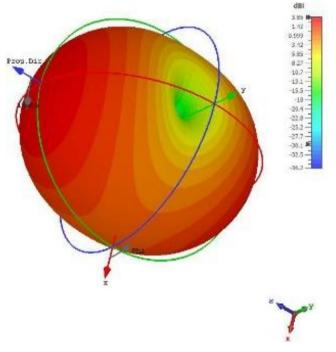
Fig. 7. Radiation pattern of the presented antenna for 2.45 GHz,
