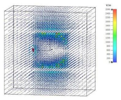
Fig. 8. E-field intensity of the proposed antenna
