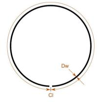
Fig. 3. The geometry of the proposed circular loop antenna
