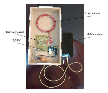
Fig. 14. Photograph of the receiver prototype (Photograph of the microwave harvesterdevice connected to a mobile phone to charge it)
