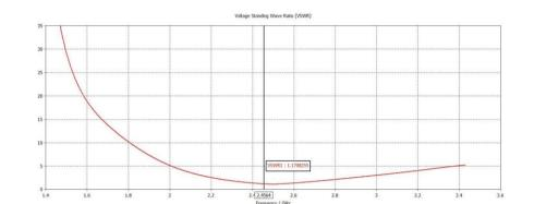
Fig. 6. Antenna VSWR vs. Frequency
