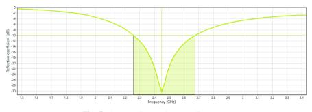
Fig. 5. Antenna Return Loss vs. Frequency
