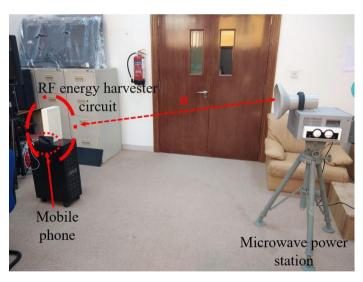
Fig. 15. Photograph of the experimental setup with a prototype
