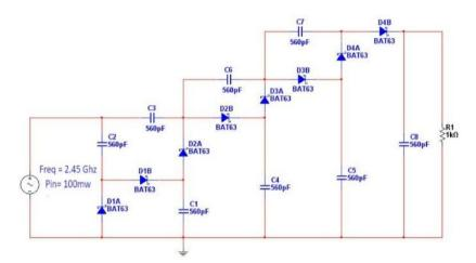
Fig. 11. Schematic diagram of microwave harvesting circuit with BAT63 diode (AgilentADS and Multisim)
