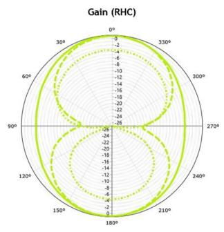
Fig. 4. Directivity of the proposed antenna
