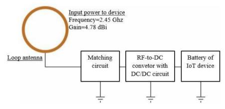
Fig. 10. Block diagram of the proposed harvester circuit
