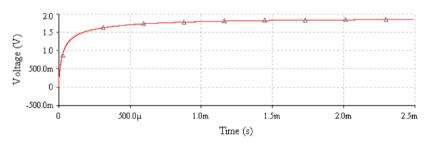
Fig. 12. Transient Analysis for 2540 MHz Charge Pump Design (100mW)
