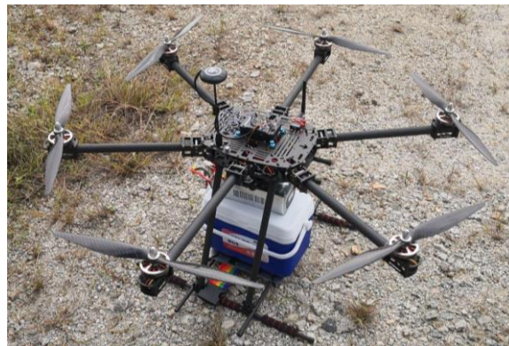
Fig. 2. Drone with cooler box for blood product delivery
