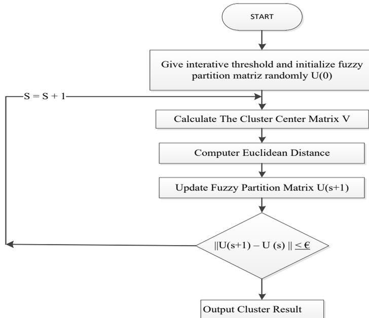
Fig. 1. The actual process of clustering using Fuzzy C-means algorithm
