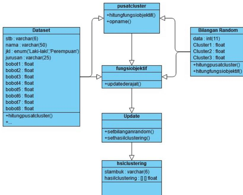
Fig. 5. Class Diagram Application
