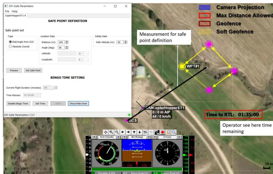
Fig. 9. Software interface for safe parameters Configuration.
