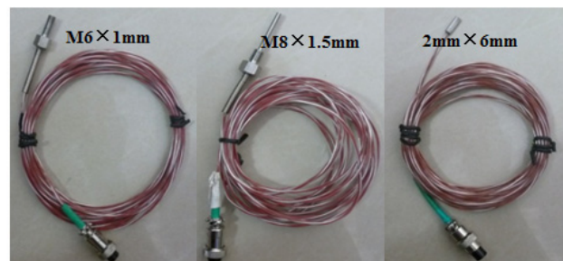
Figure 4. The thermocouples and three kinds of outer shells
