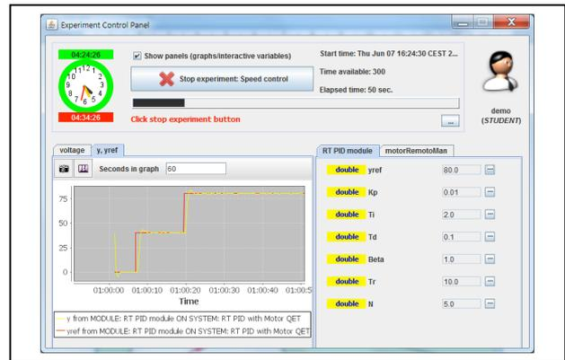
Figure 15. Experiment control panel for DC motor
