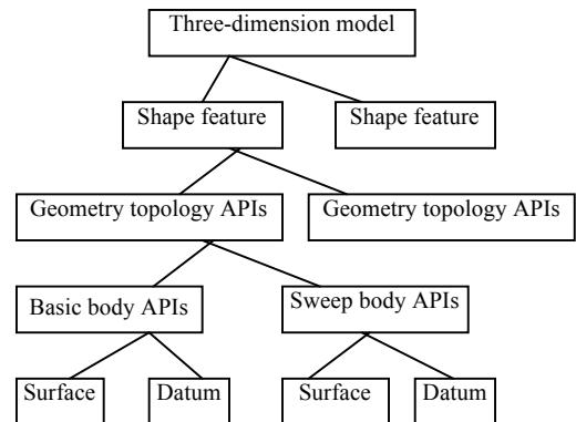
Figure 1. three-dimension model decomposition
