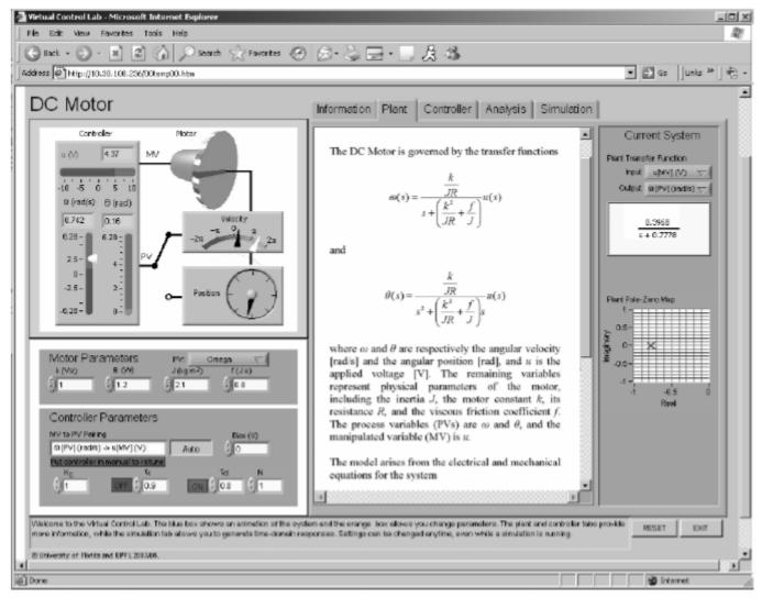
Figure 2. DC Motor Virtual Control Lab developed in LabVIEW and accessed by students using a standard Web browser [2]
