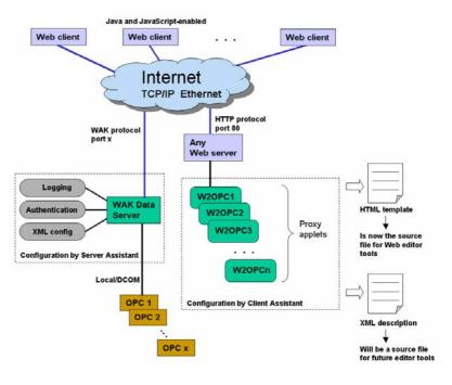
Figure 3: Component structure of the Web Access Kit for OPC
