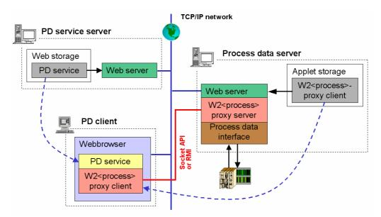
Figure 2: Distributed structure for the Web-based operation of automation devices by the LWA concept
