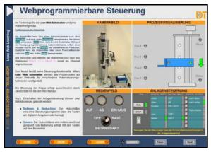
Figure 6: Remote Control of a lifting station via JavaScript
