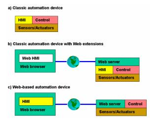
Figure 1: State-of-the-art structures of automation equipment in the Internet environment
