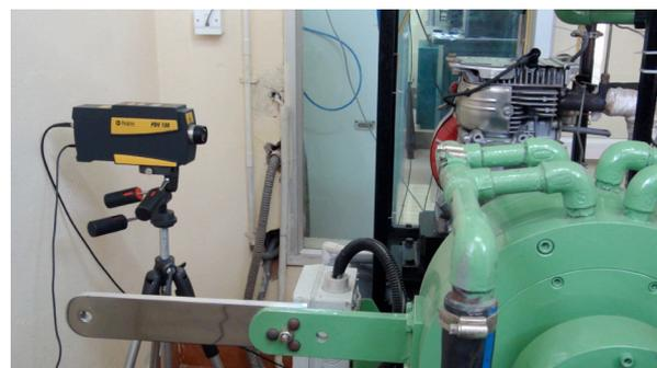
Figure 3. Laser vibrometer for engine vibration measurements
