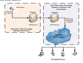
Figure 1. The working process of the new real-time video transmission approach
