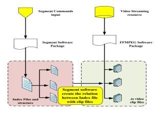
Figure 5. Segment software package working process.
