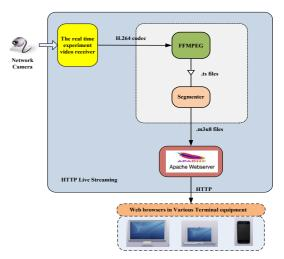
Figure 2. The architecture of the novel real-time video transmission solution.
