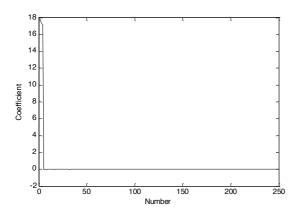
Figure 2. Coefficients of 6-level 9/7 wavelet transform of original temperature readings from sensor node 10
