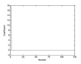
Figure 3. Coefficients of 6-level 9/7 wavelet transform after MC compression with  $\lambda = 0$  of original temperature readings from sensor node 10
