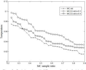
Figure 5. Deviation value with different sample ratio of original temperature readings from sensor node 10
