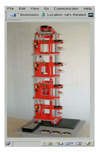
FIGURE 3: HARDWARE MODEL OF THE ELEVATOR
