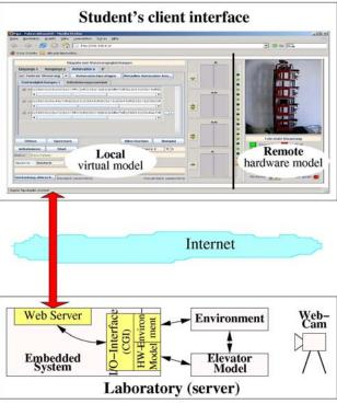
FIGURE 7: THE CLIENT-SERVER-ARCHITECTURE OF THE REMOTE LAB
