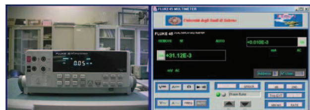
Figure 7. Real instrument and the virtual graphic interface offered to the students by SimBAD Fluke45 Service
