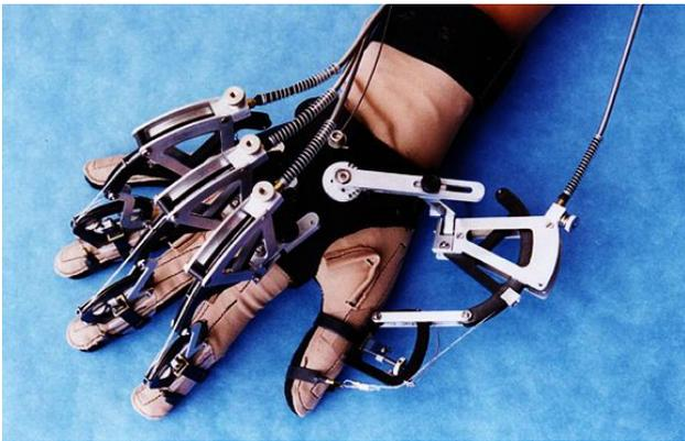
Fig. 2 Cybergrasp mechanical haptic device [6, 7]
