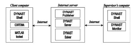
Figure 2: Environment for remote modeling, simulation and virtual experiments.
