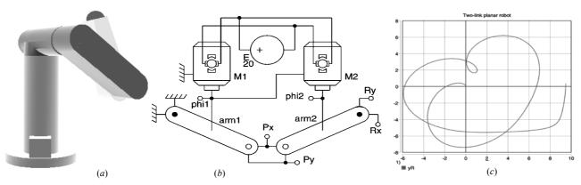
Figure 5: Robot: (a) virtual model, (b) dynamic model, (c) robot-arm trajectory.
