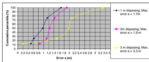
Fig. 11. CDF of the positioning error for a different disposing of the reference points from the radio map
