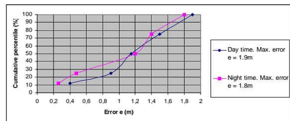
Fig. 9. CDF of the positioning error for environmental different conditions
