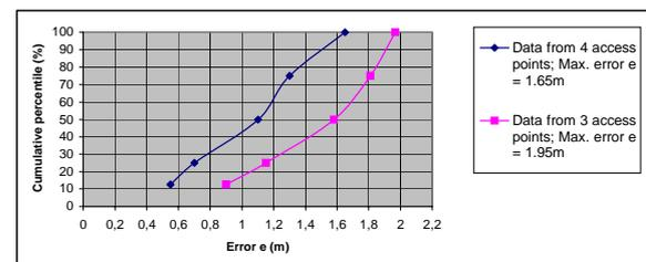
Fig. 10. CDF of the positioning error for a variable number of radio access points
