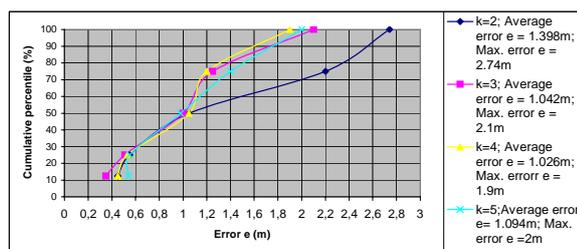
Fig. 8. CDF of the positioning error when the parameter  $k$  (the neighbors number of the first estimated reference point) is variable
