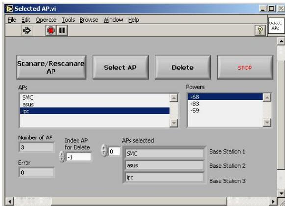
Fig. 5. The panel where are displayed all the access points scanned by the mobile user wireless card, and the received signals powers [dBm]
