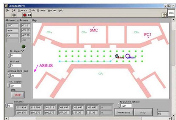
Fig. 1. The testing environment and the estimated positions of the mobile user using the average, weights and history of the last 5 positions
