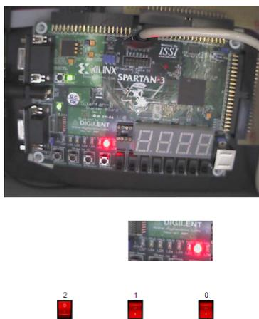
Figure 3. User's system running on a real, remote FPGA
