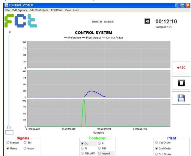
Fig. 5. Impulse response of the 2<sup>nd</sup> order system.
