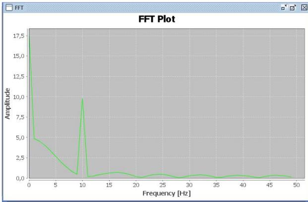
Fig. 6. Fast Fourier transform applied to a sinusoidal input signal.
