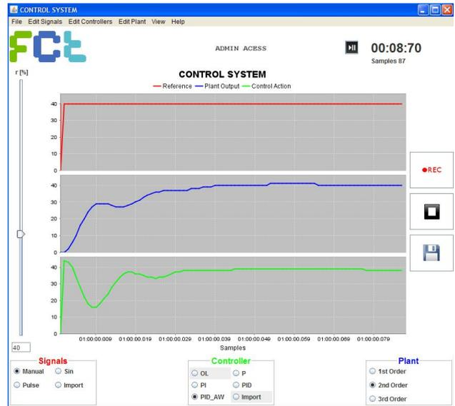
Fig. 4. Simulation result for step response, second order plant and PID controller with gains  $[K_p, T_i, T_d, N, T_t]=[1, 1, 1, 1, 1]$ .
