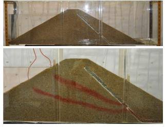
Figure 1. Small scale earth dam with a chimney drain (top); flow lines obtained with injection of color fluid (bottom).
