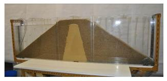
Figure 5. Small scale model of earth dam with central core, drainage blanket and toe drain.
