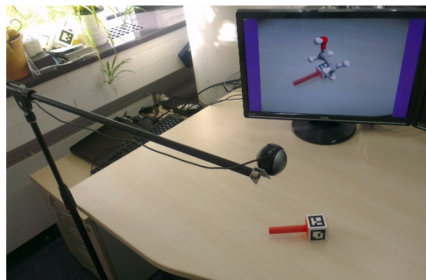
Figure 2. Computer setup for the Augmented Chemical Reactions application, using a webcam a physical cube on a handle and a monitor.
