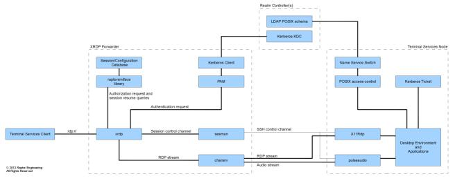
Figure 1. Architecture of the terminal services component
