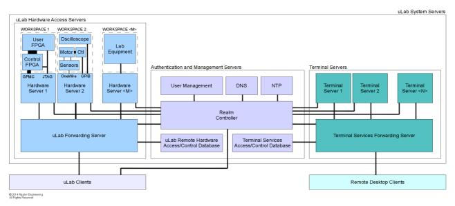
Figure 1. Major components of a generic uLab system
