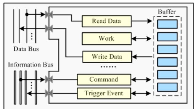
Figure 3. The function structure of instrument component
