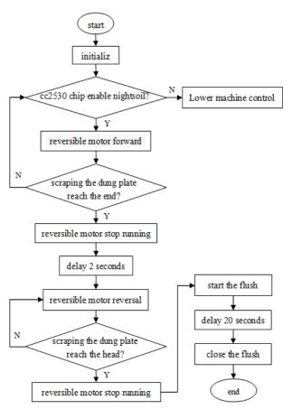
Figure 4. Manure Remover Control Flowchart
