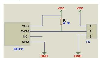
Figure 5. Temperature and humidity collection circuit
