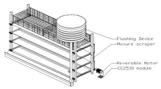
Figure 2. Structural Diagram of Manure Remover
