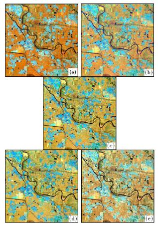
Figure 1. Original ETM+ image (RGB: band 4, band 5 and band 3)(a) and four fused images- SFIM-fused image(b), HPF-fused image (c), Brovey-fused image(d) and MLT-fused image(e)
