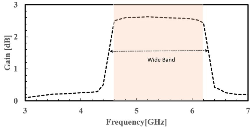
Fig. 9. Simulated gain of proposed rectangular stair step antenna
