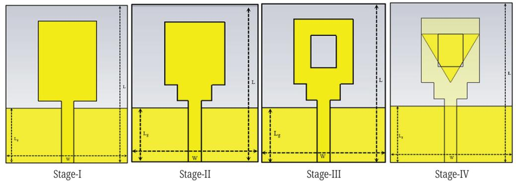
**Fig. 2.** Various successive intermediate stages of the proposed rectangular ring shape antenna
