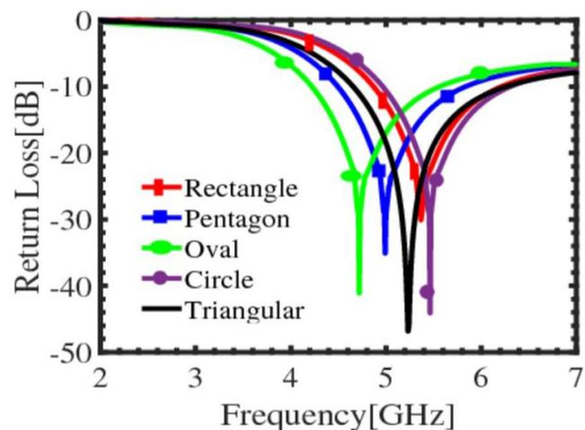
Fig. 5. Reflection coefficient of the proposed rectangular shape antenna with different DGS under stage III
