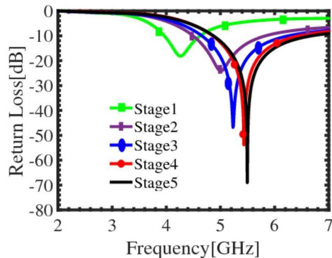
Fig. 4. Simulated return loss for different design stages of proposed rectangular shape antenna
