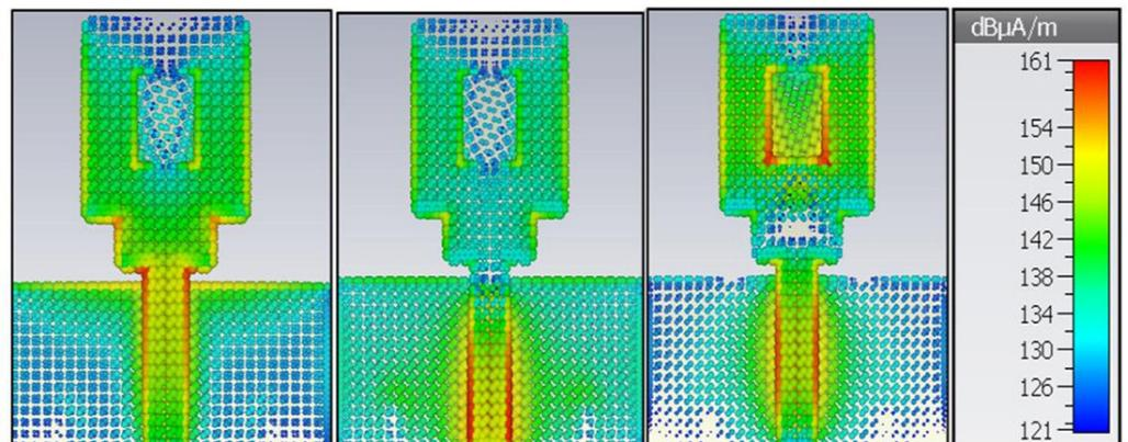
Fig. 8. Surface current distribution at different frequencies 4.6 GHz, 5.2 GHz, and 6.2 GHz
