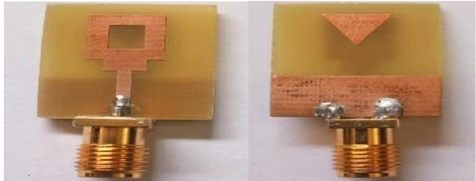
Fig. 6. Fabricated photograph of the wideband rectangular ring antenna
