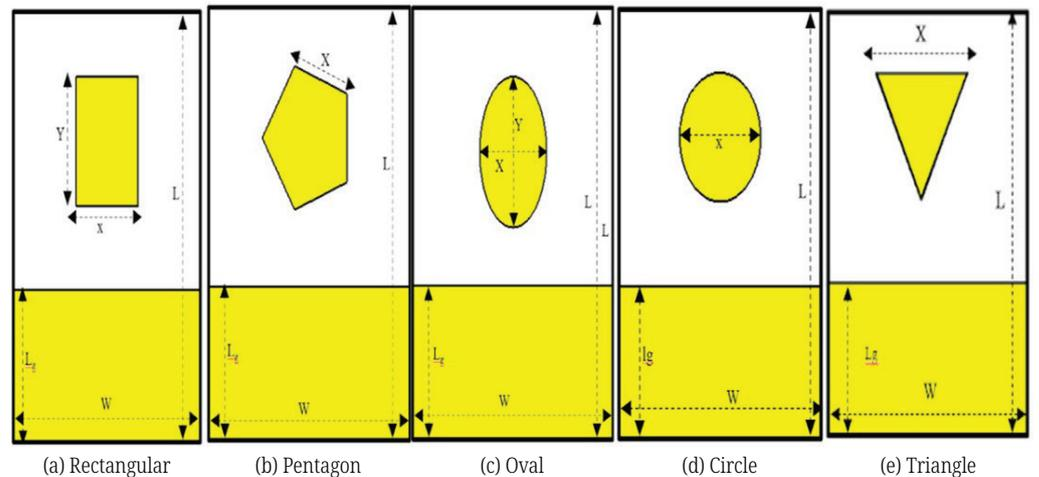
**Fig. 3.** Various DGS shapes in the partial ground of the proposed rectangular shape stair-step antenna
