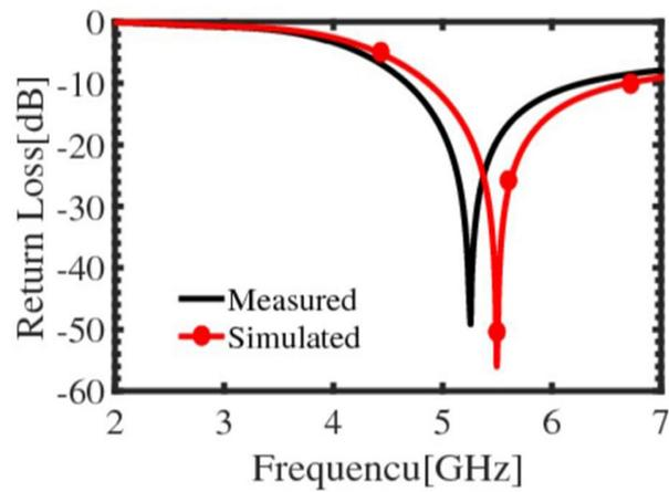
Fig. 7. Simulated and measured return loss of the proposed rectangular shape antenna
