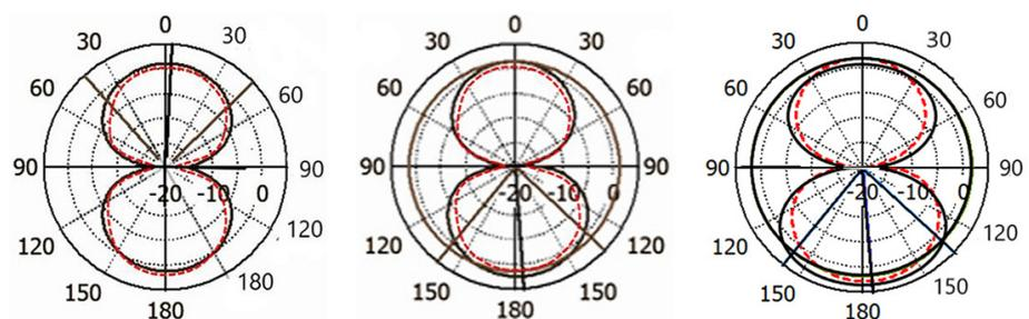
Fig. 10. Measured and simulated radiation pattern of proposed rectangular shape antenna at frequency (a) 4.6 GHz (b) 5.2 GHz (c) 6.2 GHz
