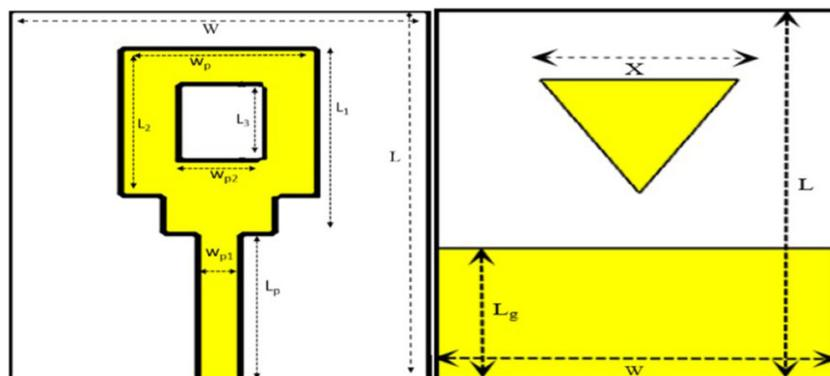
Fig. 1. Geometry of proposed wideband stair-step rectangular ring antenna
