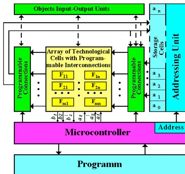
Figure 2. Block diagram of  $S_U$  for practical purposes
