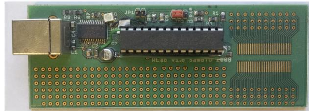
Figure 5. The RRL PCB for  $T_{MS}$  designed in accordance with the structures shown in Figures 2 and 3
