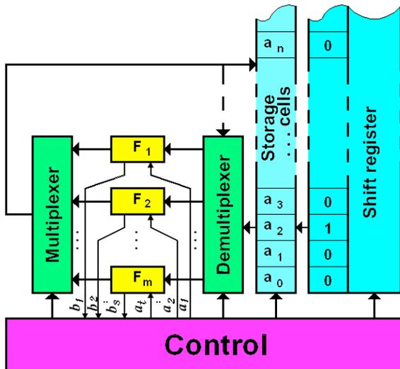
Figure 1.  $S_U$  structure of the theoretical model for the extremely multifunctional (universal) programmable synthesizer-analyzer of various objects for any formal technology  $T$
