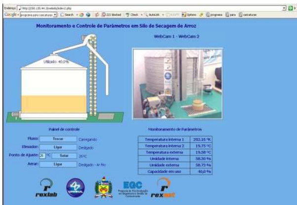
Figure 5. Web page for controlling and monitoring the silo model
