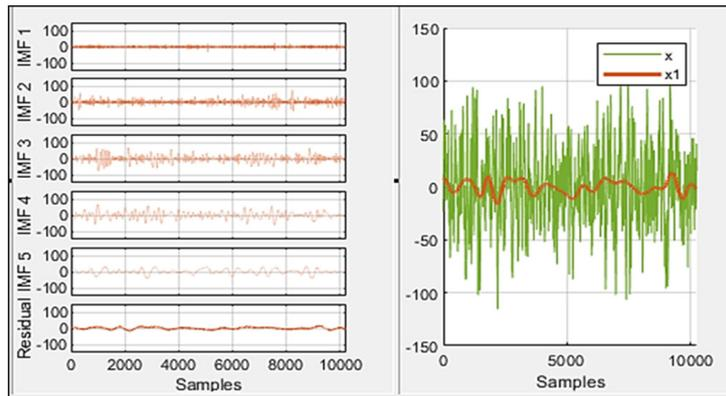
**Fig. 7.** Decomposition using EMD
