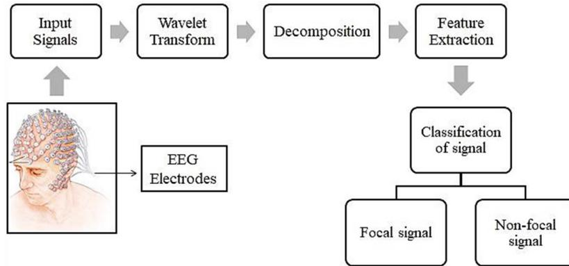
Fig. 4. Steps involved in classification of EEG signal
