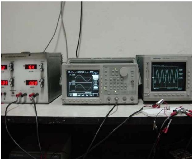
FIGURE 4. Experimental Setup of Non-Inverting Amplifier
