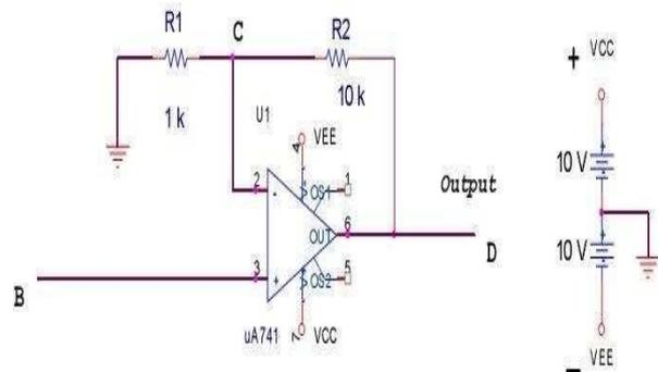
FIGURE 2. Non–Inverting Amplifier
