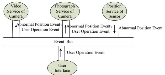
Figure 4. Architecture of Road Manhole Covers Monitoring System
