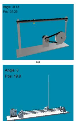
(b) Figure 10. Snapshots of virtual experiments. (a) Ball and beam control system. (b) Inverted pendulum system
