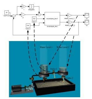
Figure 6. Interconnections between the mathematical model and 3D model for a coupled tanks test rig
