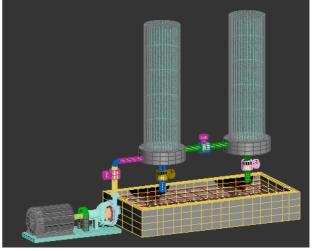
Figure 3. 3D model of a coupled tanks test rig in 3DS Max
