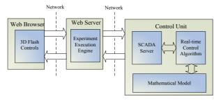
Figure 7. Structure of the data link between the 3D Flash Control and real-time simulation
