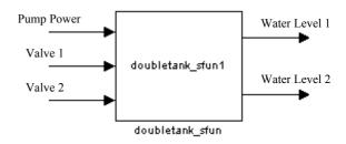
Figure 11. S-Function module for the coupled tanks mathematical model
