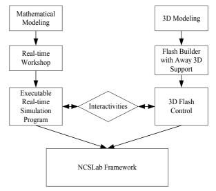
Figure 9. Design and implementation flow of a specific virtual experimental process
