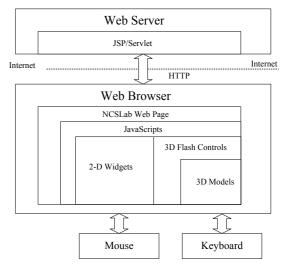
Figure 5. Structure of 3D web-based interface
