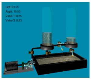
Figure 4. Virtual coupled tanks test rig rendered using Away 3D Engine with two interactive valves
