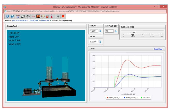
Figure 8. Web-based 3-D virtual experimental interface for coupled tanks test rig
