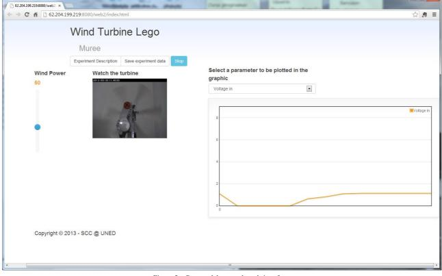
Figure 5. Remote laboratory's web interface.
