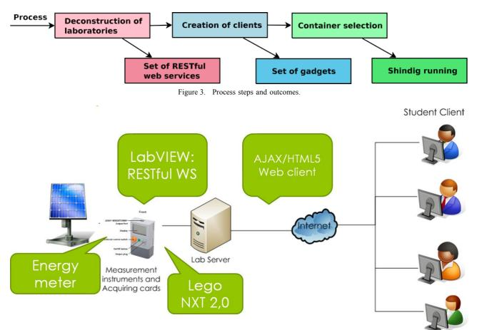
Figure 4. Structure of the low cost remote laboratory.
