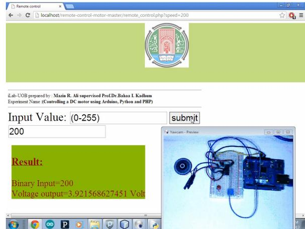
Figure 6. A mock-up of the user interface for remote control of the DC motor.
