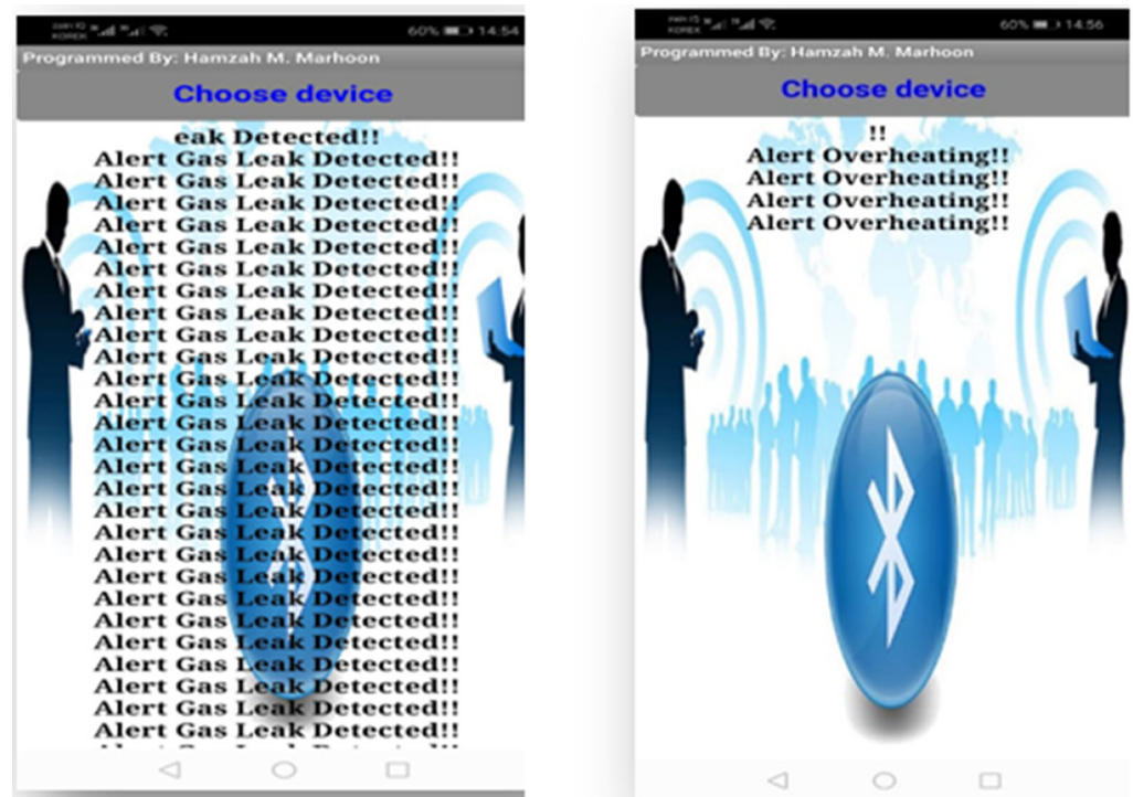
Fig. 11. Received notifications for the programmed app via the Bluetooth to the driver's phone
