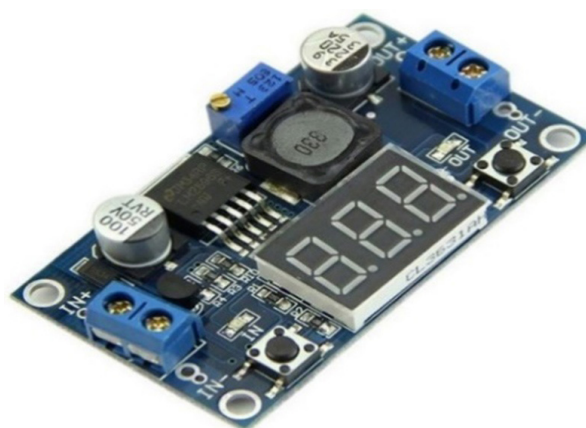
Fig. 3. A step-down voltage converter from 12 to 5 volts
