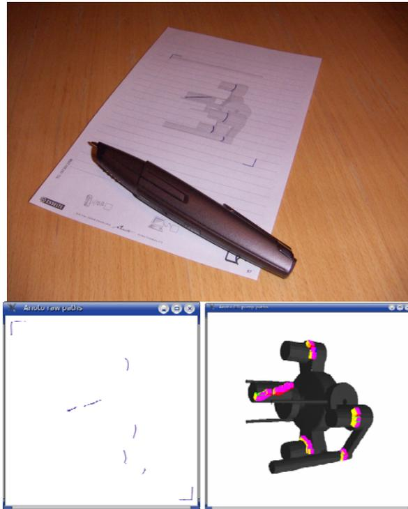
Figure 8. Foundry workpiece experiment. In upper picture the pen with the CAD model of the foundry workpiece printed on the paper enabling the Anoto technology and the pen strokes specify the cuts to be made. In the lower part, the imported pen strokes (left) and the surface mapping on workpiece 3D image.
