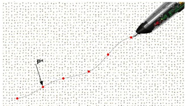
Figure 2. Sample line stroke: P\* contains position, time, status and stroke properties information
