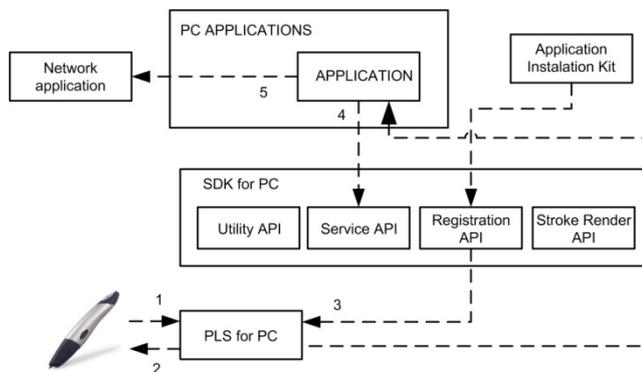
Figure 3. The PC architecture used by the digital pen [2]
