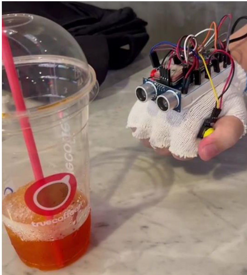
Fig. 10. Performance of gloves for helping the visually impaired to inspect obstacles
