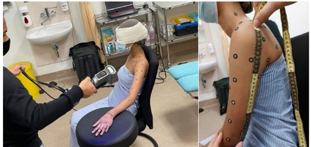
Fig. 1. 3D scanning and measurement process of the patient's left arm
