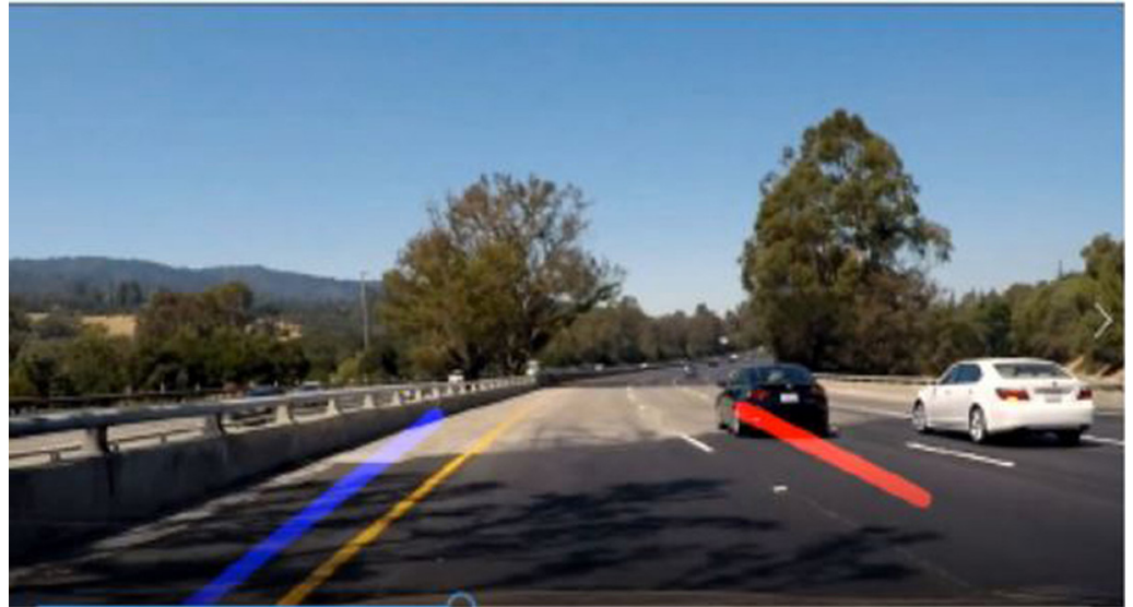
Fig. 7. The identification of lane lines can be rendered inaccurate due to shadow patterns
