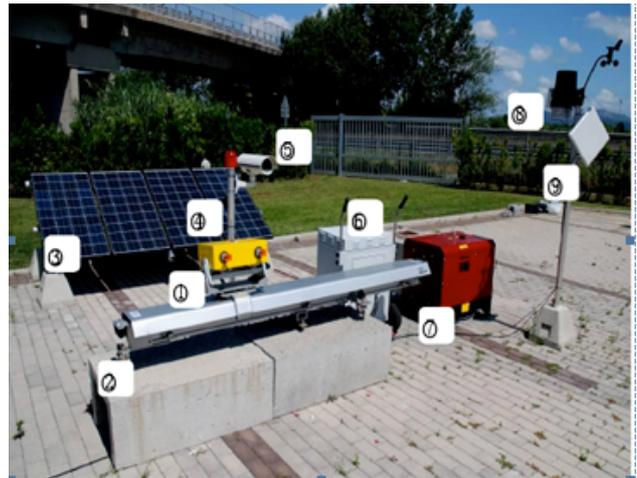
Figure 2. Ground-based SAR
