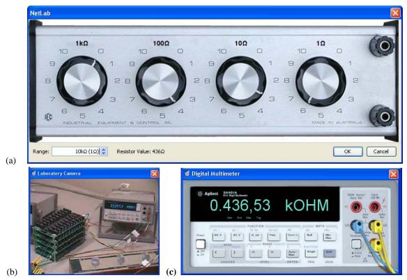
Figure 2 Variable Resistor (a) remote client GUI; (b)camera view of programmable hardware; (c) remote measurement of set resistance.
