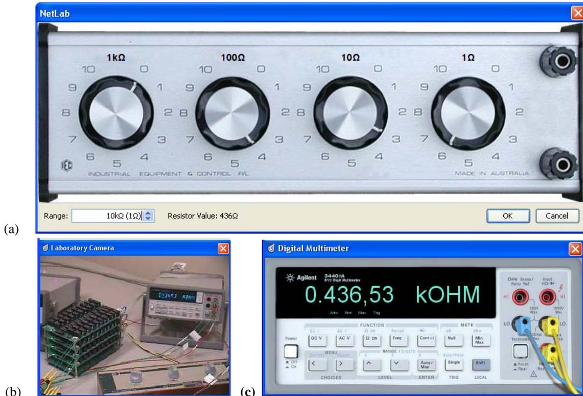
Figure 2 Variable Resistor (a) remote client GUI; (b) camera view of programmable hardware; (c) remote measurement of set resistance.
