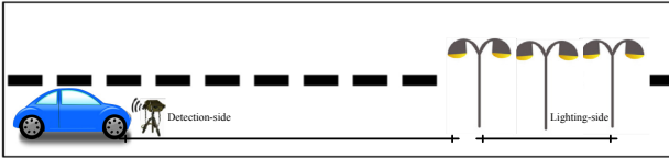
Figure 1. The idea of smart safety-lightning system
