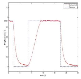
Figure 6. Arbitrary displacement control (with amplitude of 0.932in) in remote SMA experiment
