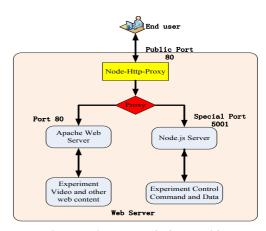
Figure 2. The new data transmission working process
