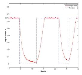
Figure 7. Arbitrary displacement control (with amplitude of 0.646in) in remote SMA experiment
