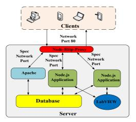
Figure 1. The architecture of the novel real time experiment control commands and data transmission
