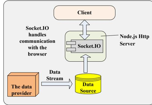
Figure 5. Socket.IO Working Process
