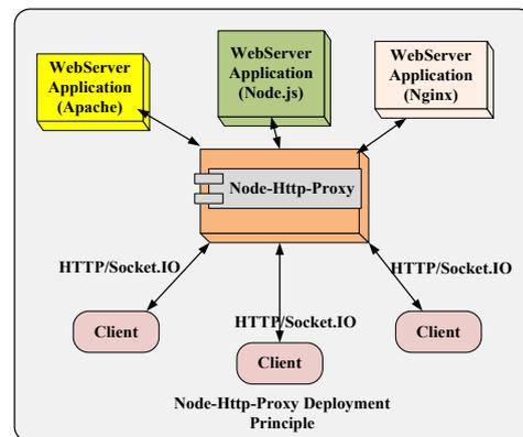
Figure 3. Node-HTTP-Proxy Deployment Principle
