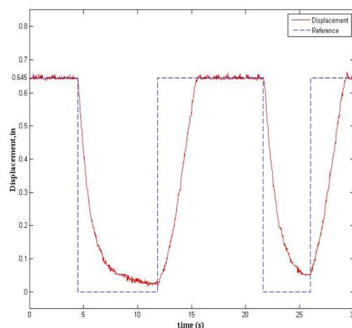
Figure 7. Arbitrary displacement control (with amplitude of 0.646in) in remote SMA experiment
