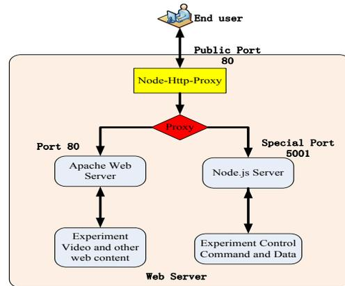
Figure 2. The new data transmission working process
