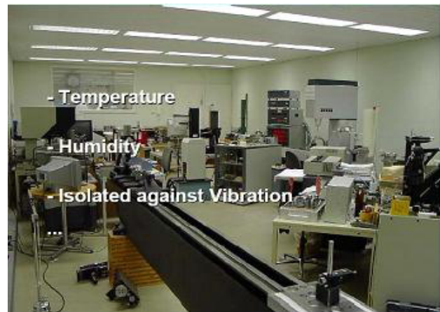
Figure 4. High precision measurement room – Nanometrology Laboratory of Vienna University of Technology
